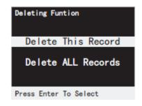
7.14.10 Press "Enter" on YES to confirm deletion or no to return to the upper interface. If yes is selected the tool will show "RECORD DELETED" as confirmation. Press "ESC" to return to the upper interface.
