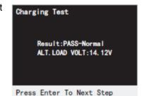
7.12.6 Press "ENTER" button to enter the next step; According to the above interface content, turn off the vehicle engine and press the "ENTER" button to enter the next step.
