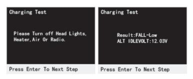
7.12.2 Then press "ENTER" button to enter the next step; The next screen is as follows: Operate the vehicle as prompted
